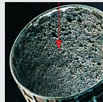
Damage caused by oil aging
