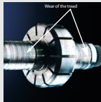
Shaft damaged by erosion
